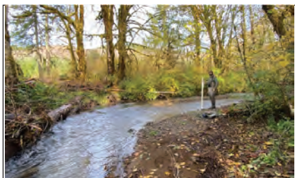
Project Manager Aubrey Cloud measures bed elevation above a large wood placement along the Luckiamute River.
