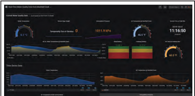
A screenshot of the real-time data dashboard at Maxfield Creek showing current water level, air and water temperature, barometric pressure. https://realtime.luckiamute.net
