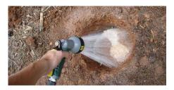
**Step 2: Fill Hole with Water ...** fill the hole with water, and let it sit overnight. This saturates the soil and helps give a more accurate test reading.
